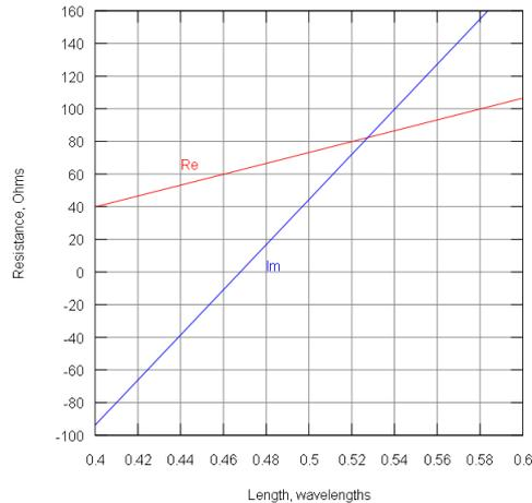
Figure 2: Impedance of a dipole [7].
