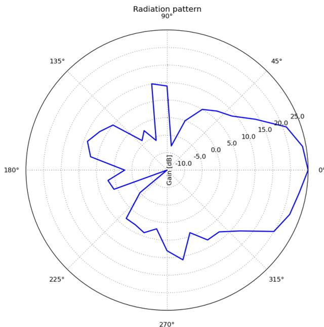
Figure 3: Radiation pattern of our Yagi antenna.
