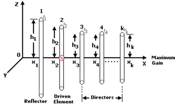
Figure 1: Yagi antenna with  $k$  directors [2].
